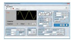
The signal generator can be programmed remotely via the USB (virtual COM) interface using SCPI commands. B&K Precision also offers application software (available for download at www.bkprecision.com) that provides virtual front panel emulation, allowing users to remotely control their instrument without the need for programming.
