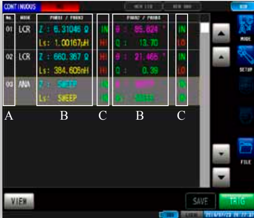
A: Panel numbers set for continuous measurement; B: Measured values; C: Parameter judgment results
